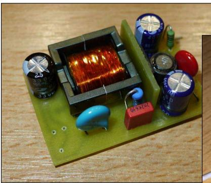
Dimensions: 33x50x12mm Power: 12 W Vout = 24 VDC Iout = 0,55A Mode: CVCC
