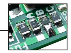
Output current ripple reduction: adding capacitor across LED string (1 uF on module). Note: capacitor will not affect operating frequency and efficiency, but it will increase startup delay and reduce maximum dimming PWM frequency. Using ceramic capacitor may result in audio noise during PWM dimming depending on PWM frequency.
